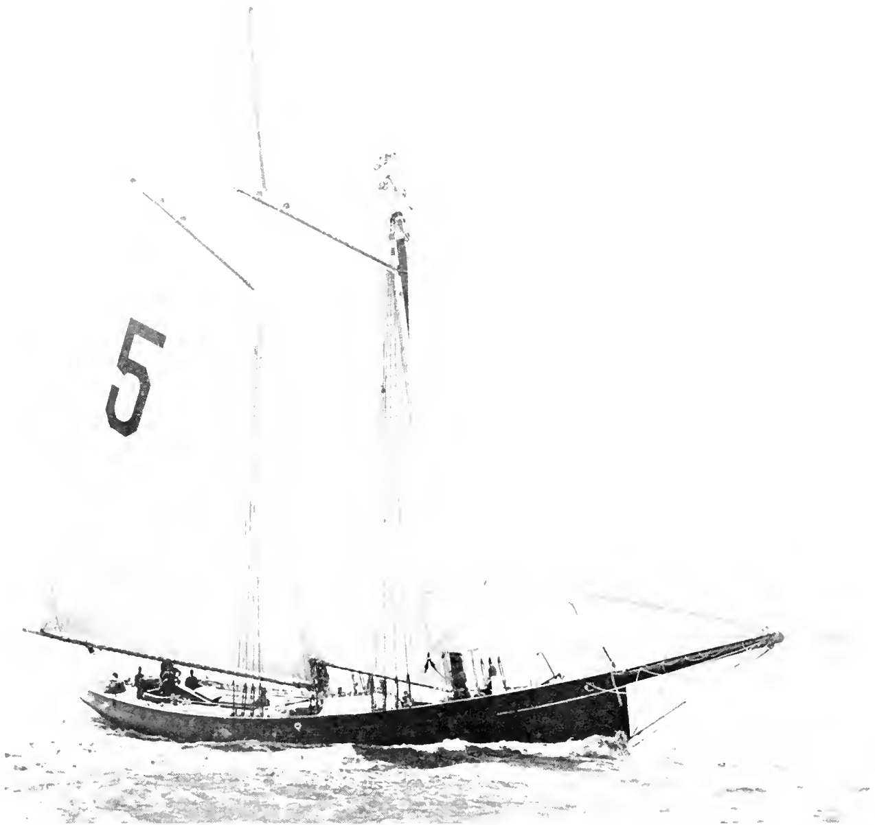
BOSTON PILOT SCHOONER Hesper , built at Chelsea, Massachusetts, by Dennison J. Lawlor, in 1884. Her register dimensions were 92' x 22' x 12', 98.94 gross tons. She is represented in the Watercraft Collection by the builder's half-model (USNM 76037; see p. 91). (Smithsonian photo 37747-b.)
